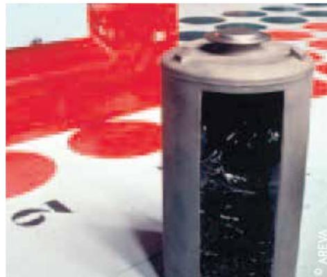
Figure 2 – Vitrified high-level metallic waste container
